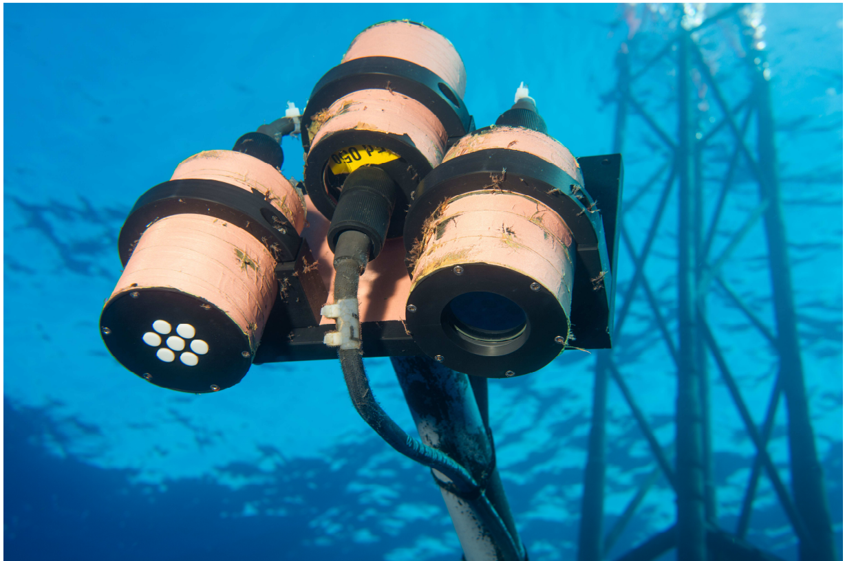
The BOUSSOLE buoy multispectral radiometers set measuring Ed , Eu and Lu at 4m depth, after cleaning by the divers.
